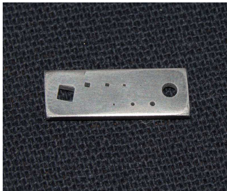
Sample of a metal part printed using the Prodways© R&D technology
