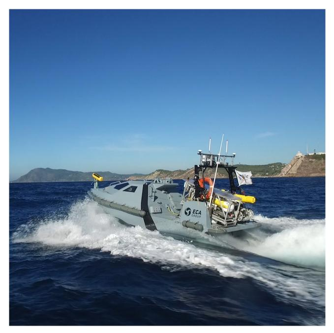
Illustration of a drone system based on Unmanned Surface Vehicle USV <u>INSPECTOR MK2</u> which can autonomously deploy underwater robots <u>SEASCAN MK2</u> (inspection robot) and <u>K-STER C</u> ( minekiller underwater robot).
