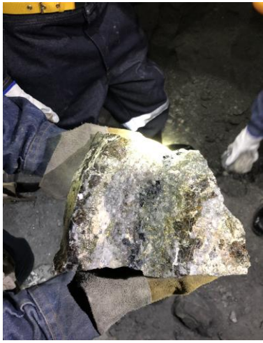
Vein sample at the El Santo Mine left to right - metallic texture: sphalerite (Zn), Galena (Pb) et Chalcopryite (Cu)
