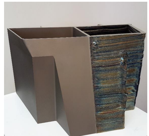
Trunk in titanium Ti64 alloy manufactured with RAF technology. Market: defense
