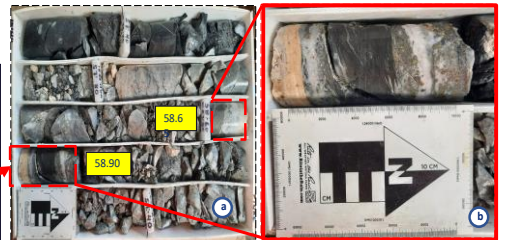
Photograph.a. (58.65 - 58.90m.) Gaby vein, made up of hyaline Quartz and altered Rhodonite with a coloform banded texture, towards the central part there is dark gray Quartzite with 1% Pyrite dissemination followed by bands of Hyaline Quartz with patches and disseminated Sulfides (Sphalerite <1%, Galena <1% and Pyrite 4%). Photograph.b. detail, Note Quartz, Altered Rhodonite and Pyrite dissemination
