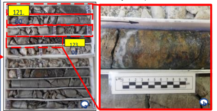
Photograph.a. (102.15 - 105.20m.) El Angel vein, consisting of a coliform banded texture vein, composed of a sequence of Massive Sulfide bands (caramelized Sphalerite 25%, Galena 20% and Chalcocopyrite <1% towards the Central part distinguishes White Quartz, Altered Rhodonite and Pyrite dissemination with moderate fracturing, followed by massive Sulfide bands (Caramel / Brown Sphalerite 12%, Galena 4%, Pyrite 10% and Chalcocopyrite 1%) with weak fracturing. Photograph.b. detail, Note the Sphalerite and Galena patches.
