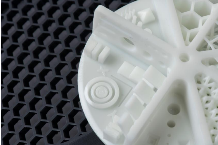
Ultra-precise parts printed with Loctite IND 475 and Loctite 3843 on Prodways' ProMaker LD 3D printer.
