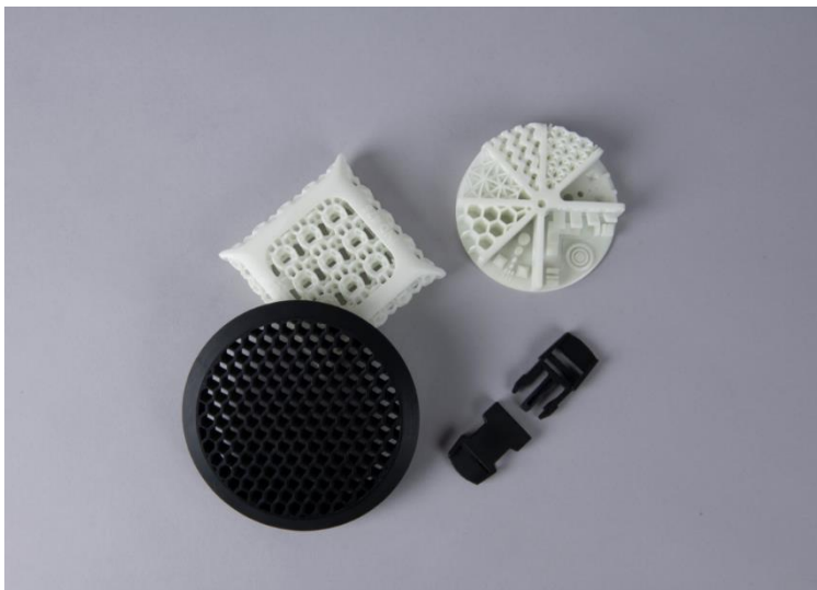
Part samples in Loctite IND 475 and Loctite 3843 printed with Prodways' ProMaker LD 3D printer.
