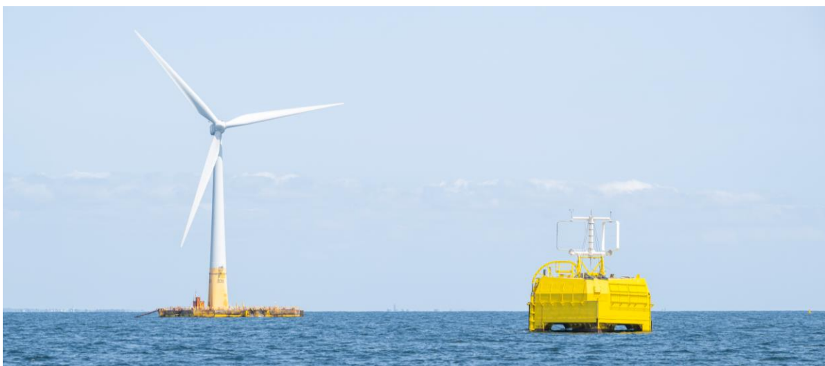
Caption: on the right : Sealhyfe offshore hydrogen production pilot (Lhyfe), on WAVEGEM platform (GEPS Techno), On the left : FLOATGEN floating turbine (BW Ideol). On the SEM-REV offshore testing site (Centrale Nantes / OPEN-C) ©Lhyfe
