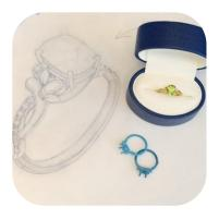
Lost-wax 3D printing technology enables jewelers to print an extremely precise wax model from a 3D digital file, with no constraints on shape, and then cast the final jewel in the chosen metal (gold, platinum, etc.).
