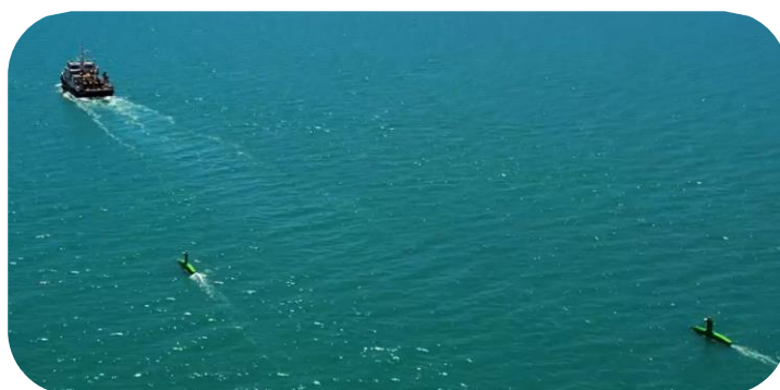
Survey operation using 2 DriX drones deployed from a traditional hydrographic vessel
