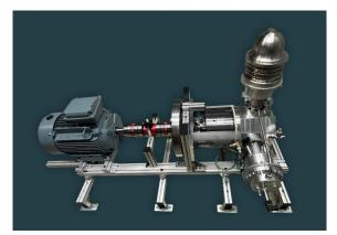
By the end of 2023, BOOSTHEAT had finalized the theoretical stage of development of the hybrid compressor, with the arrival of the first 1/1-scale prototype. The assembly of the thermal compressor and the volumetric compressor, constituting the hybrid compressor, has been completed in the BOOSTHEAT laboratory, enabling the crucial testing phase to begin.
