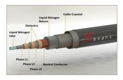
In order to reach its ideal conducting temperature, the concentric superconducting cable is cooled with liquid nitrogen. Thus it can conduct high currents with minimal loss and smaller cross-sections than an adequate copper cable (Photo: Nexans)
