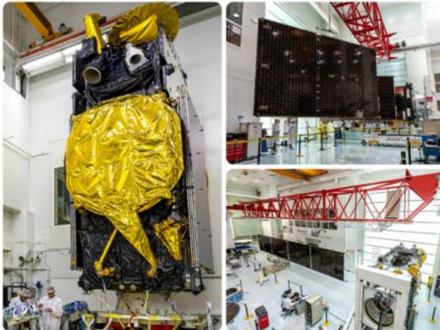
Vibration tests (left). Spreading its wings in solar array deployment (right).
