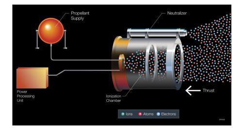
EUTELSAT 115 West B's xenon-ion propulsion system uses the force generated by a thruster ejecting electrically charged particles (ions) at high velocities. The system uses xenon as its sole propellant and the electrical energy generated by the satellite's solar panels for xenon ionisation.
