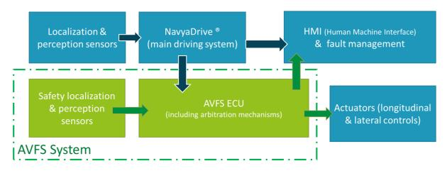
This system, composed of the NavyaDrive<sup>®</sup>, LiDAR, radar and camera sensors, associated with the AVSF computer, will be responsible for ensuring the safety of passengers and road users. In the event of an incidental situation on the route that causes the autonomous driving system to go out of its operating range, it will be able to adapt the vehicle's behavior in complete autonomy, without human intervention.
