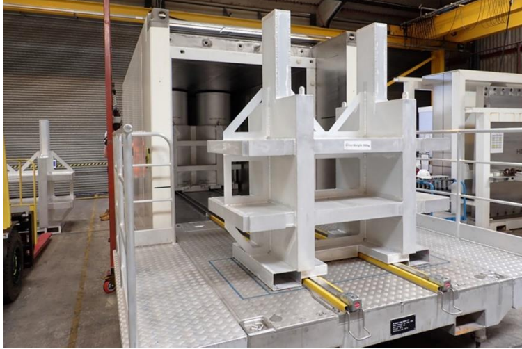
Intermediate Level Waste loaded into a TN Gemini container, copyright NWS
