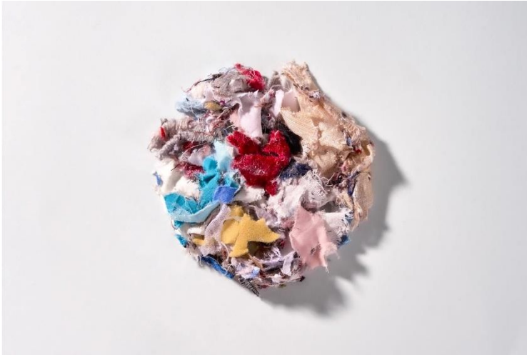
Figure 4: Textile waste leaving Carbios' preparation line, suitable for enzymatic recycling
