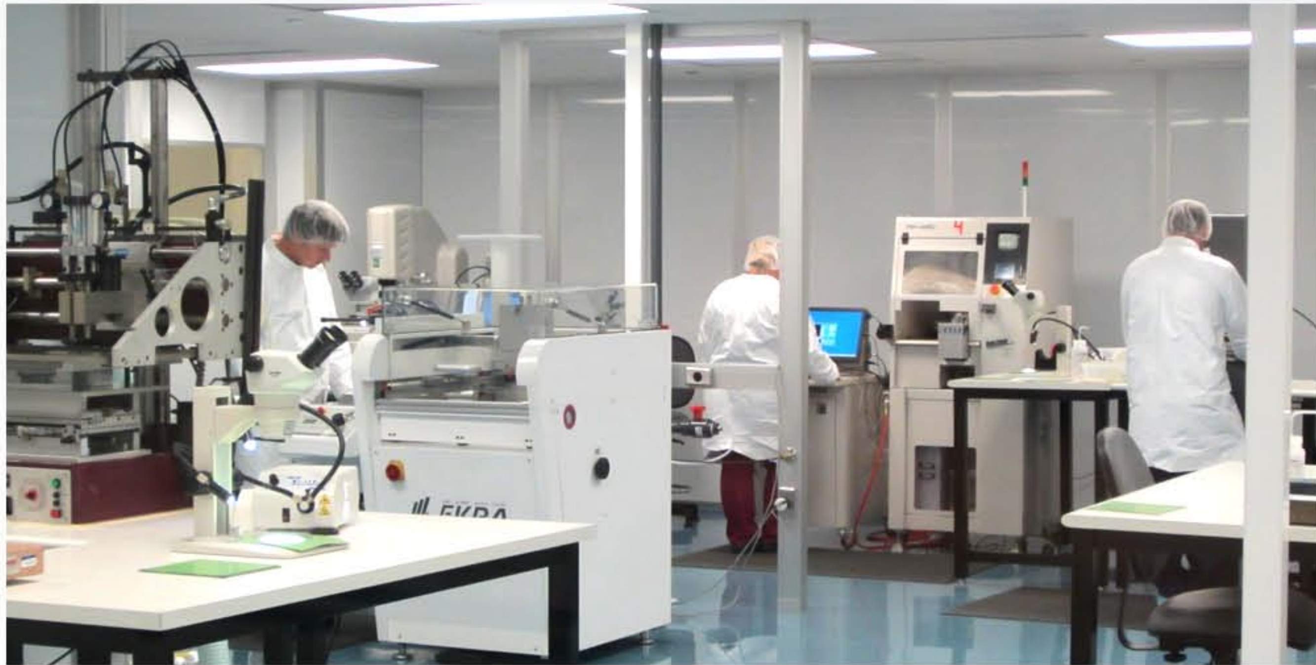
Cambridge, Maryland - 2,000 square foot Class 10,000 clean room
