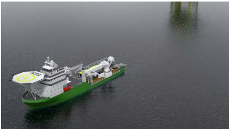
3D views from Cortez Subsea of Bourbon Evolution 800 with pipelay spread.
