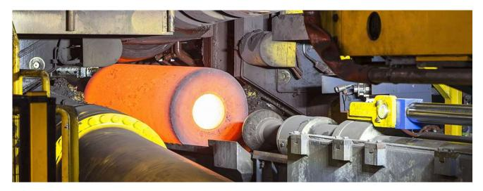
The piercing of solid steel billets and their hot rolling on a mandrel are two key stages in the production of seamless steel tubes. Controlling these processes is crucial to the dimensional and metallurgical quality of the products. With this new tool, Vallourec demonstrates its determination to maintain its highest level of technological expertise and reinforces its position as a global leader.
