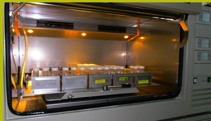
CO2 incubator "Kuhner" for the production of a few mg of antibody to be purified with a robot.
