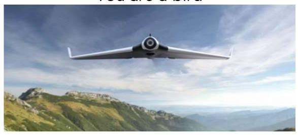
Parrot Disco is an ultra-light wing-shaped drone. Controlled by autopilot, it is very easy to fly.
