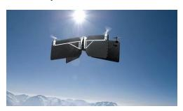
The X shape of **Swing** enables it to **fly both vertically and horizontally.**
