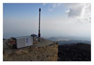
The recently deployed network linking Mount Etna on the east coast of Sicily to scientists in Clermont-Ferrand, France, 1,200 kilometers away, transmits radon measurement data, which helps scientists monitor activity of the volcano. Radon is a natural radioactive element found in high concentrations near volcanoes and uranium deposits and is one of the potential precursors of volcanic eruptions.
