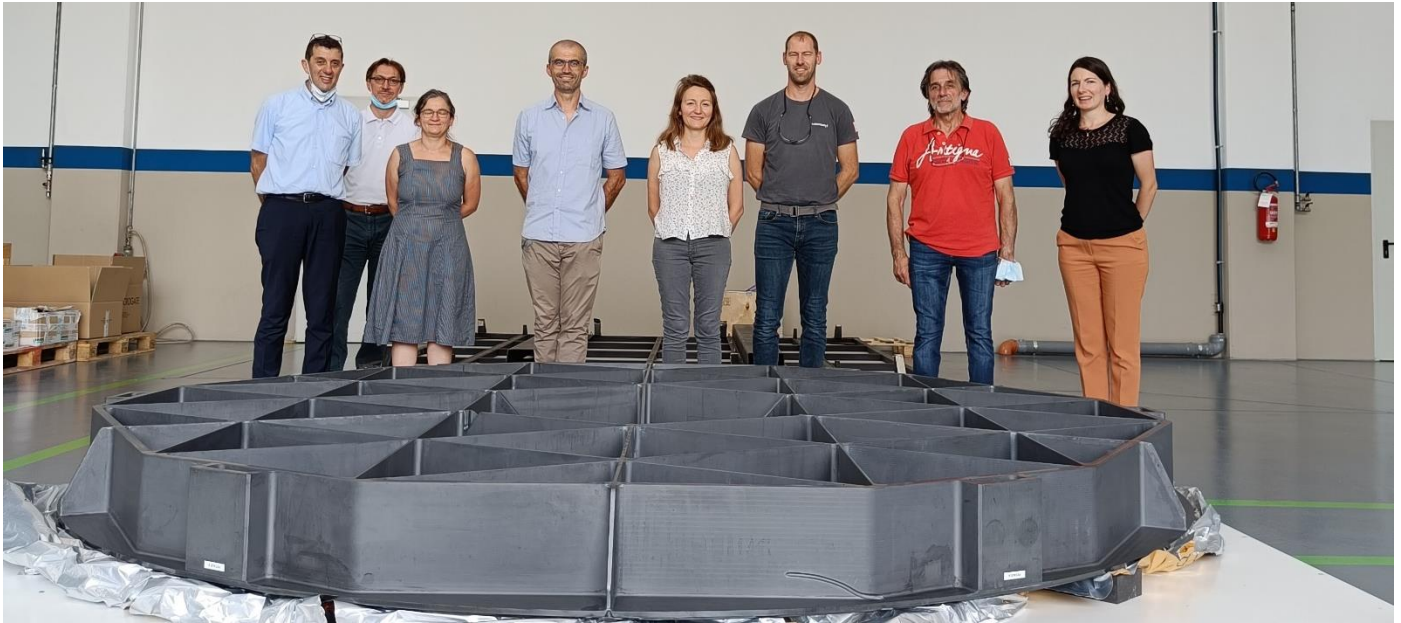
Reference Structure of the Adaptive Mirror of the ELT
