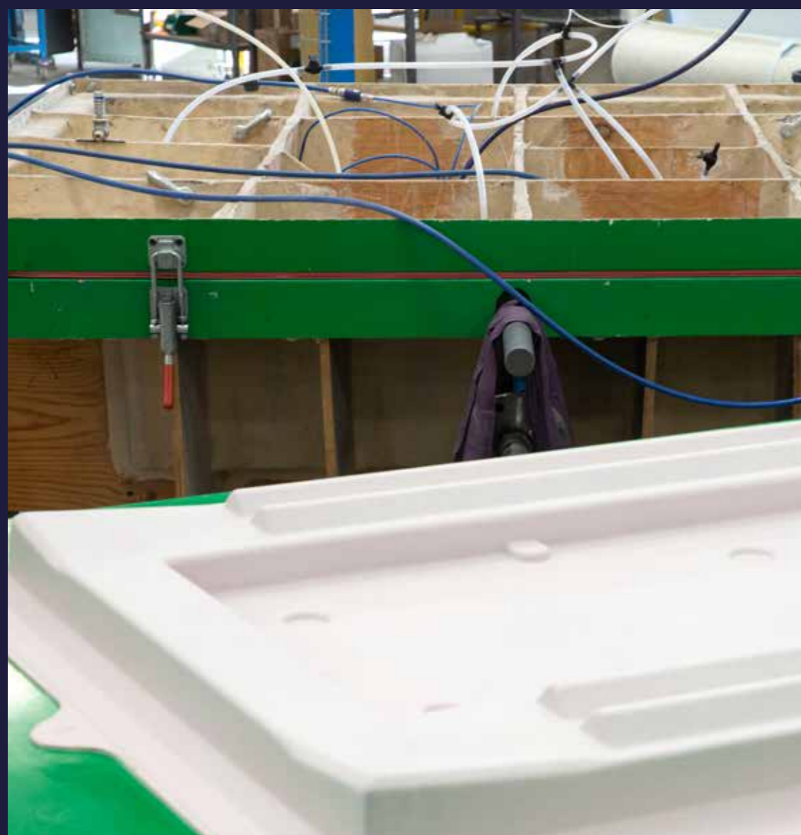
ALTHEORA Composites - Site de St Etienne de St Geoirs RTM (Resin Transfer Molding Process)
