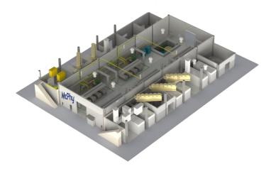
3D simulation of the 20 MW electrolysis platform equipped with McPhy technology Augmented McLyzer
