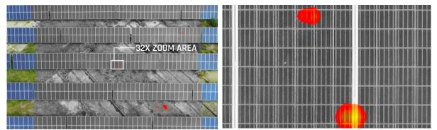
Solar panel anomalies detected with the thermal camera, before and after the 32x zoom.
