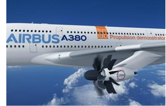
Modification of the A380 wing to test "Zero Emission" engines
