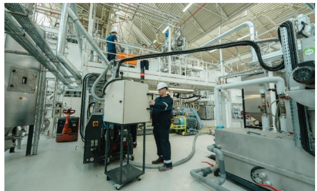
Figure 3: A production line for CARBIOS Active is already up and running at CARBIOS headquarters in Clermont-Ferrand, France, which can produce 2,500 tons/year of CARBIOS Active (required for the equivalent of 50,000 tons/year of enzyme-embedded PLA).
