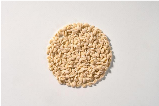
Figure 2: CARBIOS Active, in granule form, integrated directly into PLA-based packaging or products at the production phase, enables compostability at room temperature.
